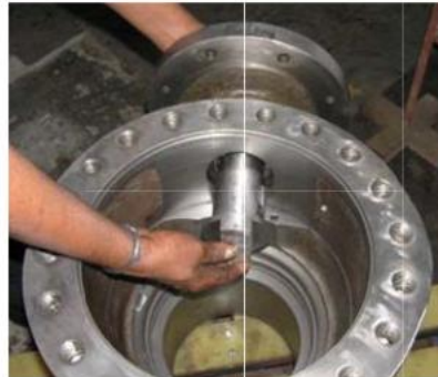
Fig.10. Stem being inserted into the body
