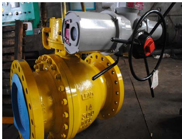
Fig. 5. YODO Valves TMBV with Gear unit & Gas actuator.
