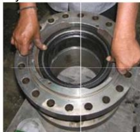
Fig.13. Seat ring being inserted into the connector
