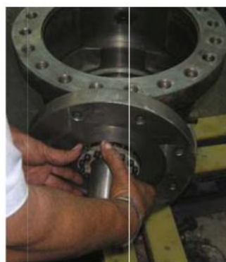
Fig.11. Gland packing inserted into the body
