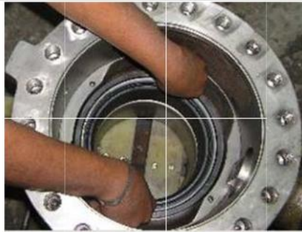
Fig.9. Seat ring assembly inserted into the body
